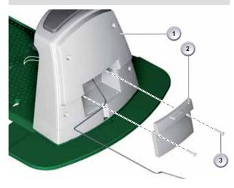
■ To check the connection, unscrew the fastening screws (3) and remove the cover (2) from the base station (1).
