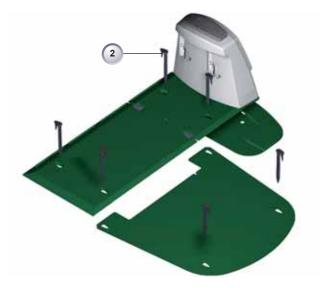
3. Connect the base station to the electrical power supply (see chapters 5.7 - 5.8 - 5.9).
